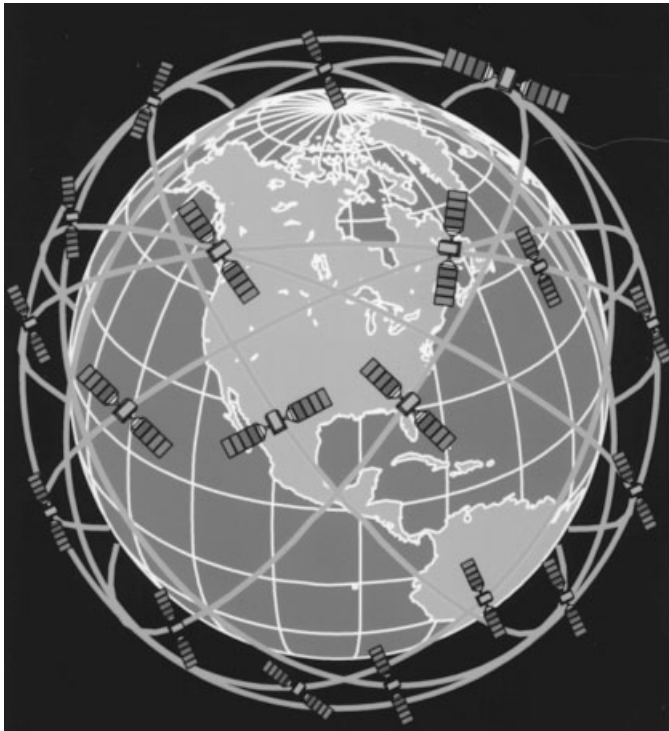
Figure 27.13 Globalstar 48-satellite constellation. (Courtesy of Globalstar.)
