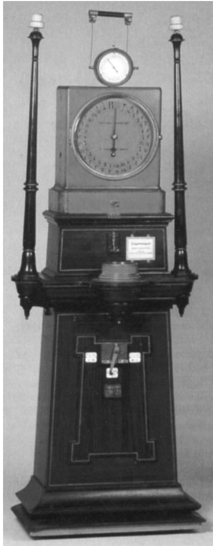
Figure 6.16 Typograph made by the clockmaker Leonhardt, 1844. (Scanned from Post- und Telekommunikationsgeschichte , Vol. 2, 2000, p. 61, with permission of the Deutsche Technikmuseum, Berlin.) See insert for a color representation of this figure.
