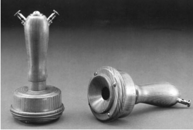
Figure 10.7 Bell's butterstamp telephone, 1877. (Courtesy of Museum für Kommunikation, Frankfurt, Germany.) See insert for a color representation of this figure.
