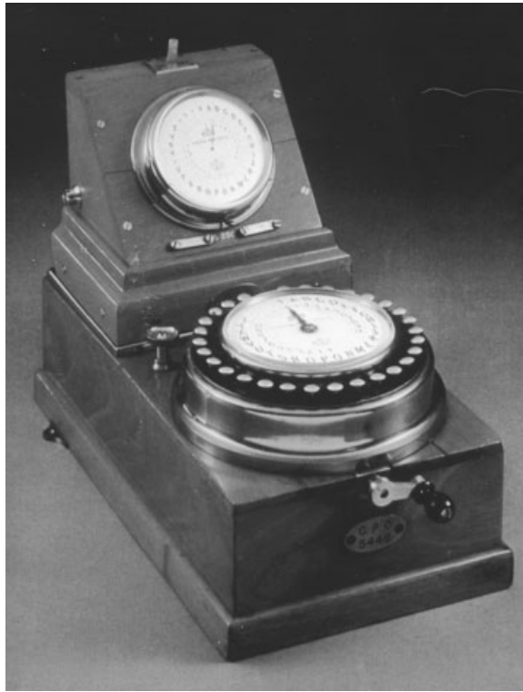
Figure 6.12 ABC pointer telegraph. (Courtesy of Museum für Kommunikation, Frankfurt, Germany.) See insert for a color representation of this figure.
