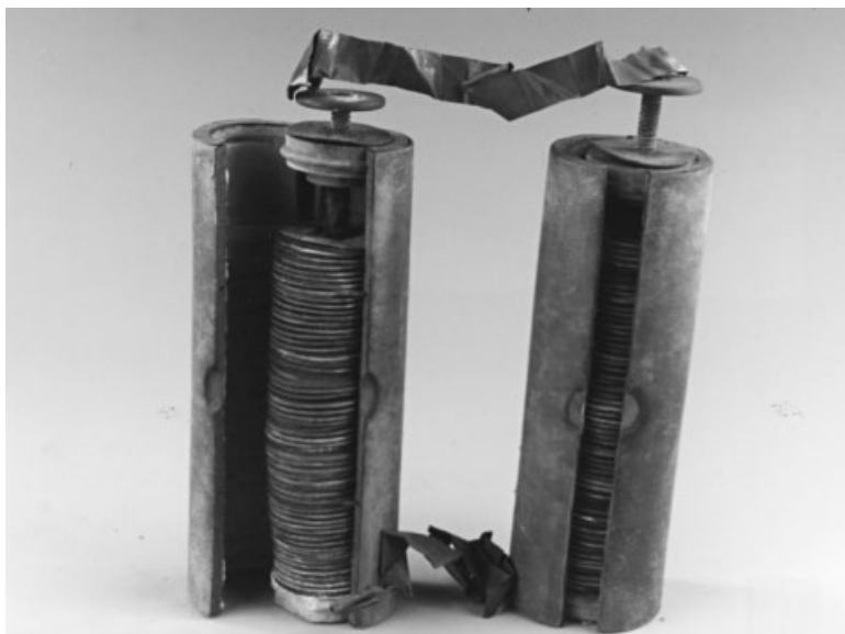
Figure 4.1 Two original voltaic piles connected in parallel. (Courtesy of Musei Civici Como.)
