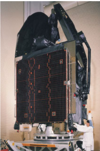
Figure 27.7 Satellite HS 601 HP made ready for launch, 1999. (Courtesy of Boeing Satellite Systems.)
